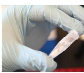
9. Place your centrifuge tube into your centrifuge and spin for 10 minutes at 13000rpm to separate the cell debris from your desired DNA (after this spin there should be cell mass plastered to your tube
