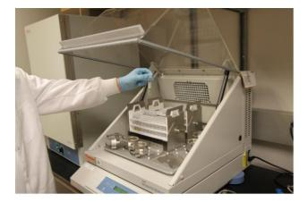
3. Drop the Pipette tip into the inoculation tube and return the tubes to your shaker incubator to grow. (estimate time of growth varies across cell types, usually between 8 and 24 hours)
