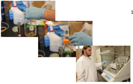
1. Using a pipette aid, carefully add 5ml of liquid media to your 15ml inoculation tube. Repeat for every colony you are inoculating. Place your inoculation tubes into your 37C shaker incubator and allow 15 minutes for the media to warm up. (if you are making a reference plate, place that plate into your incubator at this time) Remove tubes from incubator along with your plates
