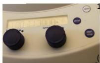
13. Pipette 750ul of Qiagen PE wash buffer to your spin column and spin for 1minute at 13000rpm. Dump the liquid that collects in the 2ml tube.
