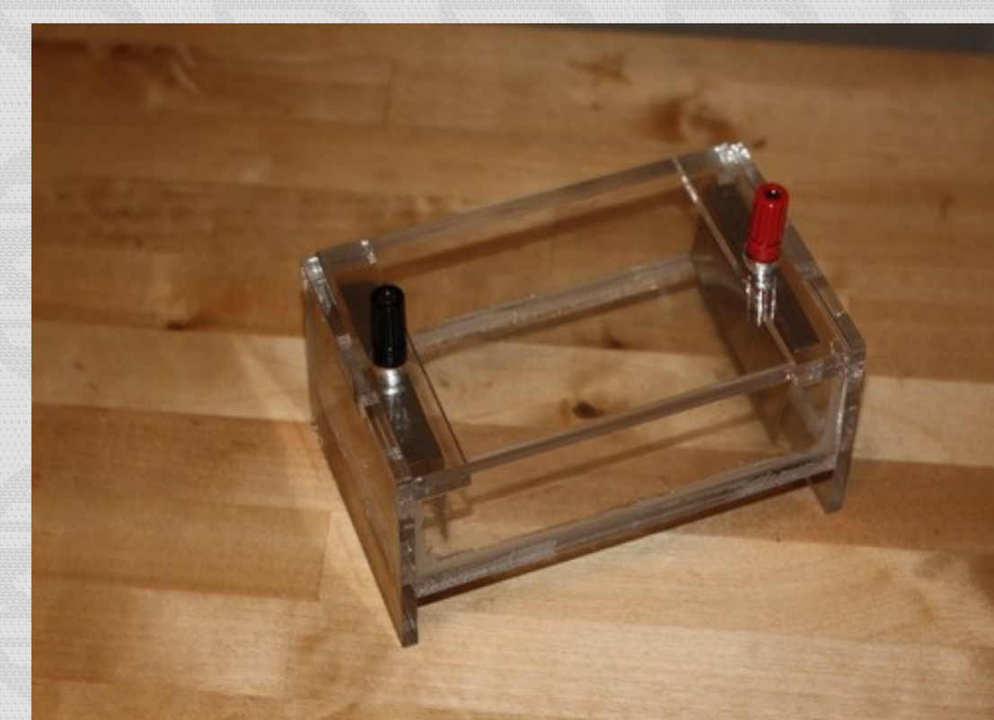
Figure 8. Horizontal gel electrophoresis box. Cost of this unit is projected to be less than $10.00
